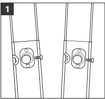
**Step 1:** Remove nuts & bolts (3) from connectors (4) on the frame (2) & keep safe.
