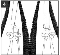
**Step 4:** Place handle (1) over the connector (4) on the frame. Match the holes on the handle & connector, push bolt through hole & secure with nut tightly.
